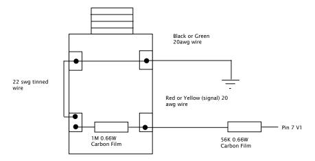
Lightly twist the black and red wires together, keep them short enough and have them away from any AC sources of noise - the input is the most important to keep free of this.
