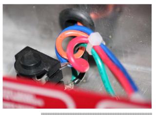
The speaker jack and O/P Tx wires before the modification.
