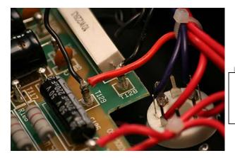
Move the red wire of the output Tx from T128 to T129 (now upstream of the output DC supply).
