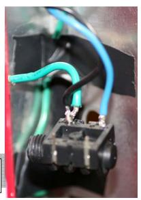
The speaker jack after the removing the power stage switch.
