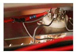
Input Jack Left: Wired Farnell Socket Right: 56K resistor connecting to pin 7 on valve 1.
