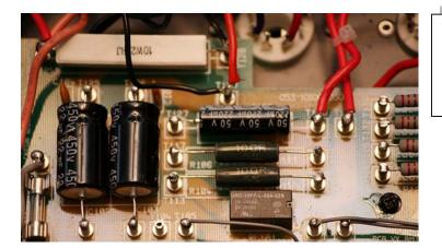
The power valve cathode resistors now are 100R/6W wire-wound, replacing the previous 120R resistors. Dave Petersen used 3W carbon film resistor.
